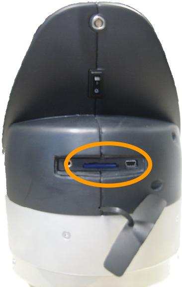
**Figure 7: SD card and USB connector**
