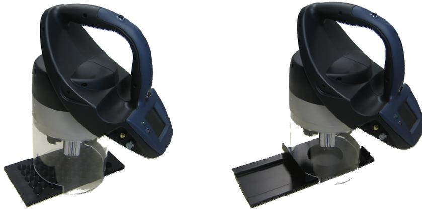
Figure 4: Accessory for grape berries (50 cells and 100 cells)
